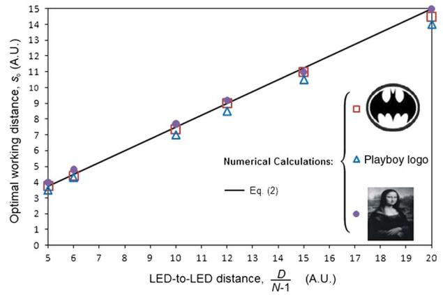
Fig. 4. (Color online) Optimal illumination distance in function of the separation between two adjacent LEDs. Shown here are the linear fitting [Eq. (2)], and numerical results using three different target images. Each numerical point is obtained using the method described in Fig. 3 for Lambertian LEDs. Batman logo is a trademark of DC Comics and is used with permission.
