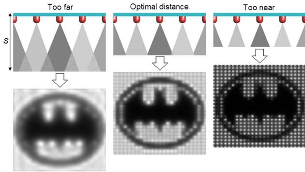
Fig. 2. (Color online) Concept of optimal working distance. If distance  $s$  is too long, the light pattern is blurred; and if it is too short, the pattern becomes a hot-spot distribution. Note that LEDs are modulated with the optimal intensities that require each of these three working distances. Batman logo is a trademark of DC Comics and is used with permission.
