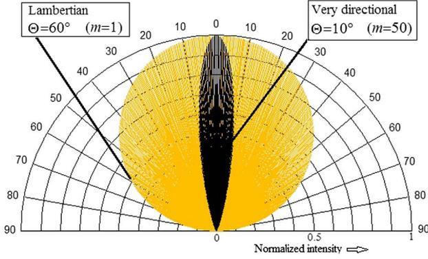
Fig. 5. (Color online) Radiation pattern of an LED with the cosine-power model [10]. Here  $\Theta$  is the half-width at half-maximum (HWHM) angle.
