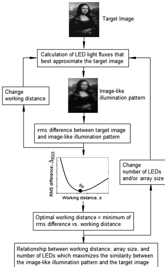
Fig. 3. Methodology used to find the optimal relationship between the illumination distance, LED array size, and number of LEDs. In this letter I consider only square grids (Fig. 1).
