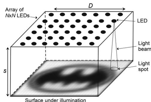
Fig. 1. LED array producing an image-like illumination by modulating the intensity of each LED. Here  $s$  is the working distance,  $D \times D$  is the array size, and  $N \times N$  is the number of LEDs. Batman logo is a trademark of DC Comics and is used with permission.
